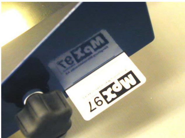
The Smart-card is inserted in the slot on the right side of the display. Make sure that the contact points are turned towards the back of the monitor.
