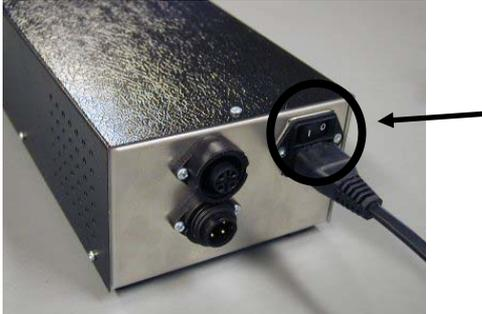
Use the switch to turn the unit on/off.
